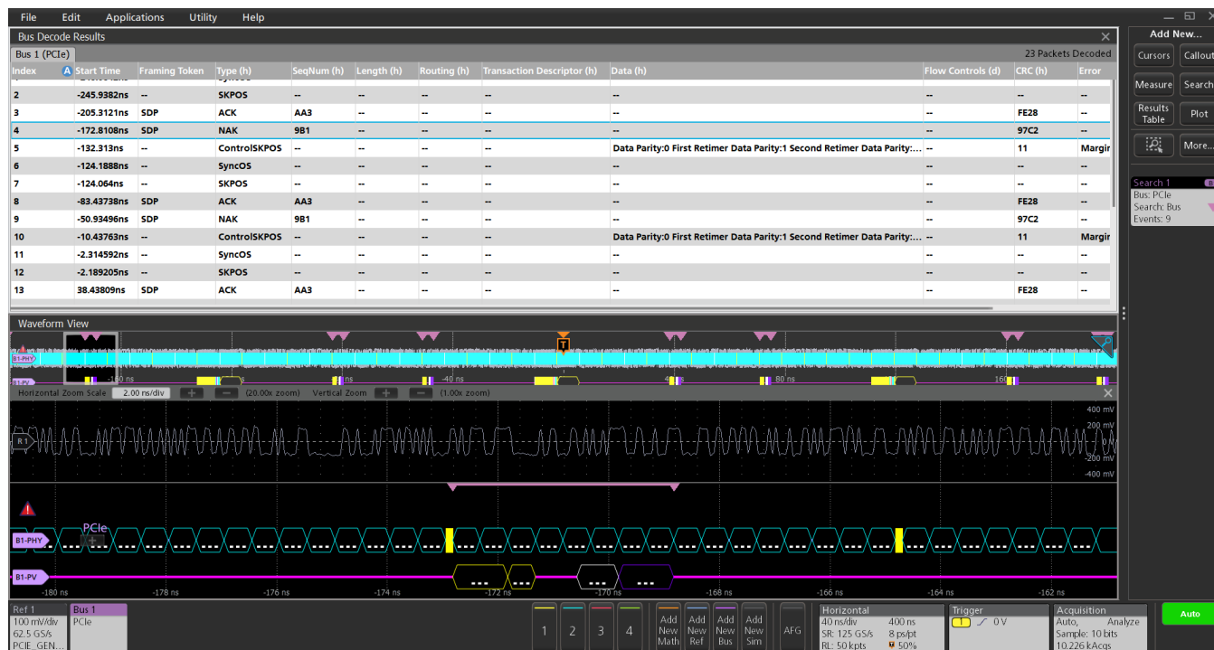
Triggering on a PCIe Gen4 high-speed serial bus with decoded packet display.
