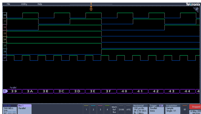
With color-coded digital waveform display, groups are created by simply placing digital channels together on the screen, allowing digital channels to be moved as a group.
