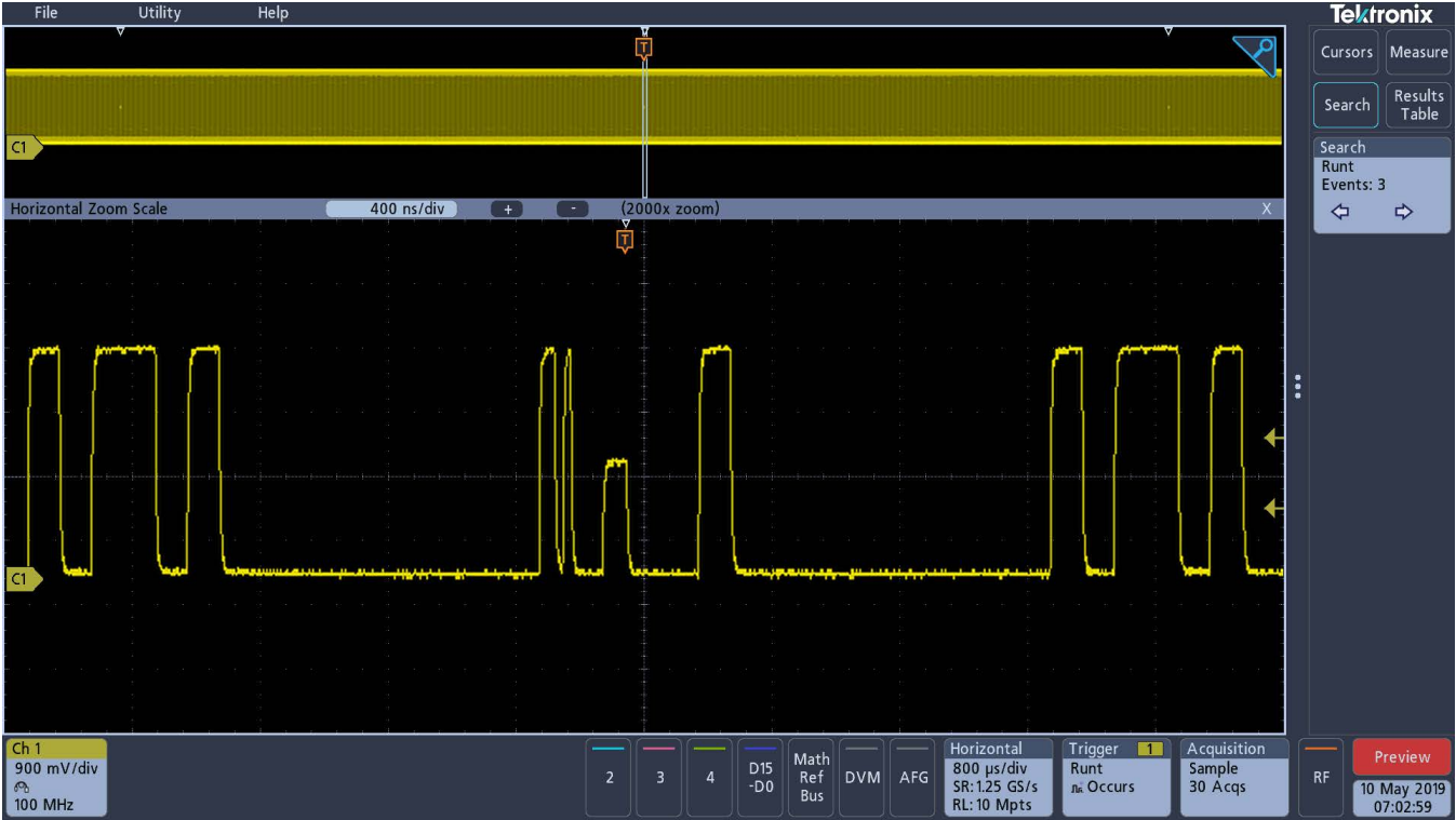
FastAcq helps with revealing the presence of runt pulses in the digital data stream for further investigation. In this test case, Search revealed and marked 3 runt pulses in the 10 Mpoints acquisition.
